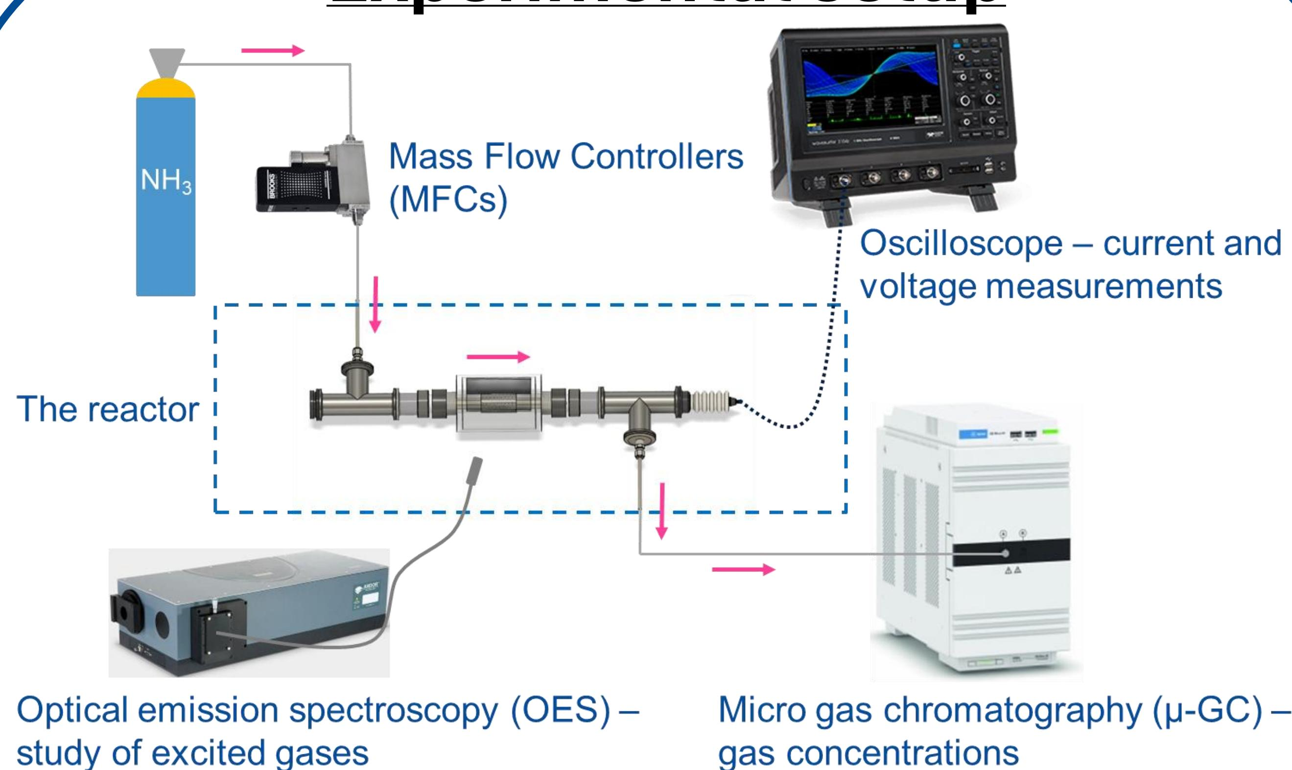
High concentration of ammonia is fed into the dielectric barrier discharge reactor, where it is converted into hydrogen and nitrogen by the plasma. The outlet gases are analyzed by micro gas chromatography (μ-GC) to determine the ammonia conversion.
