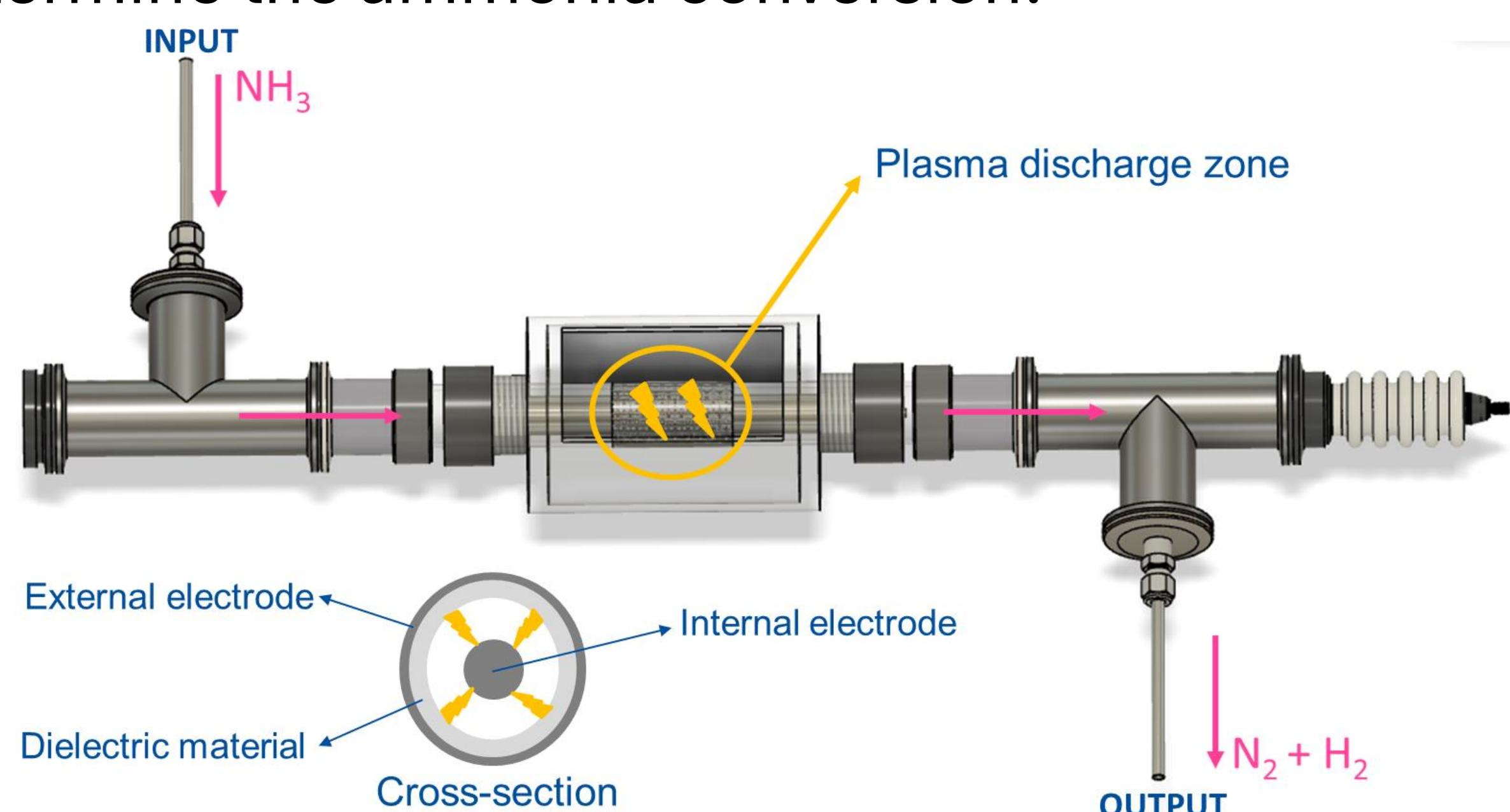
Plasma is generated by applying a high-voltage signal between the two electrodes, one of which includes a dielectric material. The resulting discharge is performed at atmospheric pressure and room temperature, and can be characterized using various diagnostic techniques, such as optical emission spectroscopy (OES) and oscilloscope measurements.
